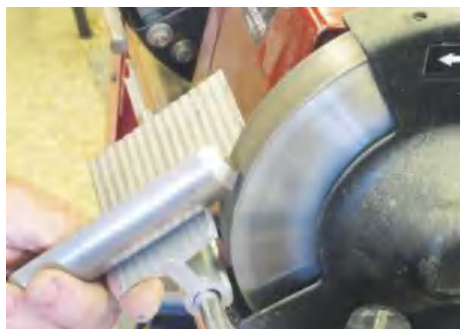
▲ Pic.2 The tool is best sharpened using a platform to set the angle. Placing marker pen on the bevel will show if you are grinding the correct angle
